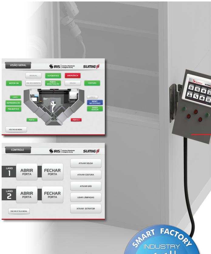
1 *Screen that allows you to view information about a program, welding efficiency, current and voltage.*
